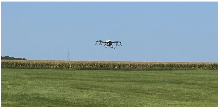
This is an example of a commercial drone used for pesticide application on agricultural fields. Photo credit: Butler SWCD.
